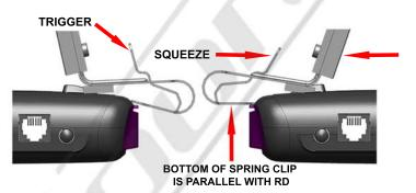
2 - The bottom of the spring clip must be parallel with the top of the RD to slide in and out. SLIDE THE RD ONTO THE SPRING CLIP AS FAR AS IT WILL GO. Release the trigger to secure the RD onto the mount. Before installing the mount onto your rear view mirror, remove and install the RD a few times so you can observe how the spring clip functions.
