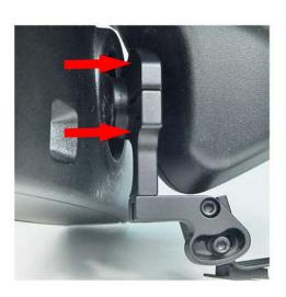
4 - Position the mount as far forward as you can. Before fully tightening the clamp screw, make sure the bottom of the mount is parallel with the bottom of the mirror.
