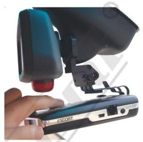
6 - To access the buttons of the RD you will need to gently push downward on the front of the RD with one finger and push the desired button with another finger. Then allow the RD to return to it's original position by gently letting it spring upward. When accessing the buttons, be sure to push the RD downward just enough for your finger to fit between the RD and mirror. Do not push down more than what is needed.
